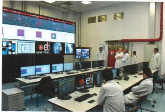
Figure 1. The ELI–NP laser control room during the first experiment. The wall screen is showing the HPLS state machine, live diagnostics of the laser, vacuum control, environment monitoring, experimental area and target live view.
